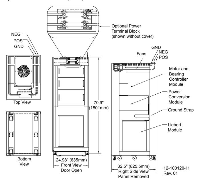
Figure 134Liebert FS cabinet mechanical installation
